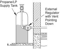
Figure 12 - External Regulator With Vent
